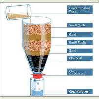
Use a pant leg or cone shaped object and fill with charcoal from your fire and two alternating layers of clean sand and small rocks.
